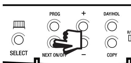
4. Continue programming the central heating **ON** and **OFF** times in this way by using the **+** or **-** buttons to set the time you want and pressing the **NEXT ON/OFF** button to move to the next setting.
