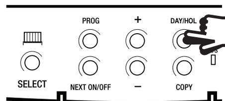
6. Press the **PROG** button twice to return the unit to **RUN** mode (time appears and the colon in the display begins to flash).
